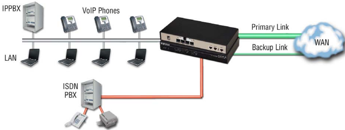
Figure 7. WAN uplink redundancy
